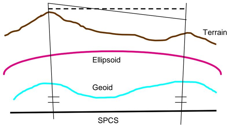
In New Jersey, the surface of the State Plane Coordinate System is approximately 640 meters below the surface of the ellipsoid along the central meridian.
